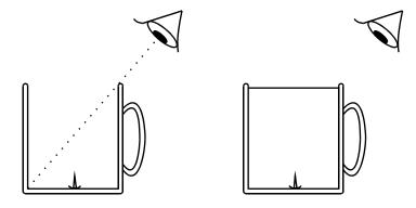
The first beaker is empty. The eye cannot see the drawing pin. The second beaker is full of water and the eye can see the drawing pin.
